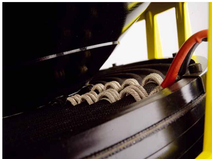
Soldered-on leads and 2 x 3 thick tinsel leads per coil
