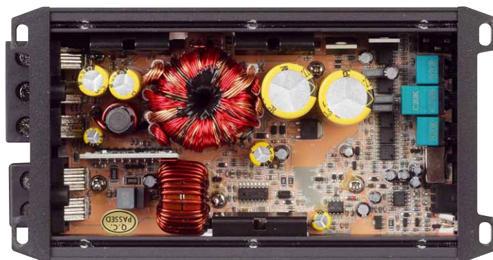
The SX-ONE features a robust power supply and a generously sized toroidal transformer behind the amplifier stage
