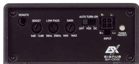
The mono version has a bass boost and a low-pass filter
