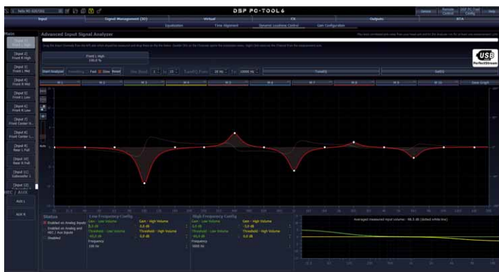
The inputs now feature 15 EQ bands, time correction and the dynamic loudness (DLC)
