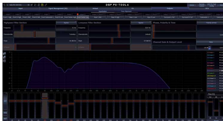
All 16 outputs come with crossovers, EQs, delay, phase and level adjustments
