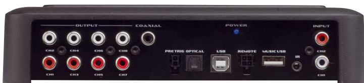
The ZDA has 8 processed outputs if the power amplifier section is not needed
