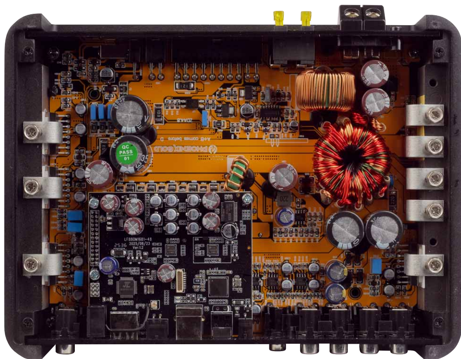
DSP on a daughter board, four analog amplifier ICs mounted on the outside of the heatsink
