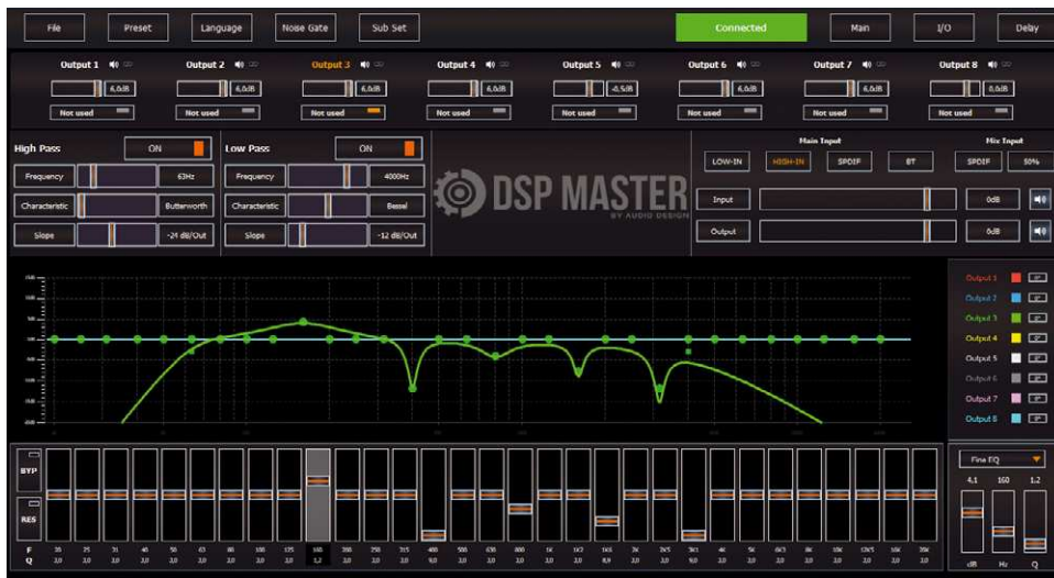
The main window features SPL, crossovers, and 31 EQ bands for the channels
