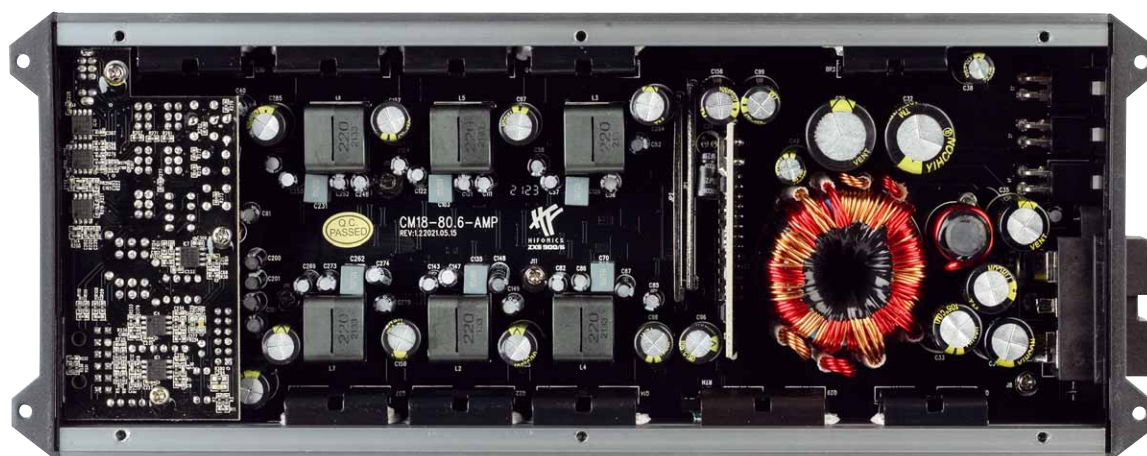
Neat layout featuring only the large components on the visible side of the circuit board; the driver chips are positioned on the rear
