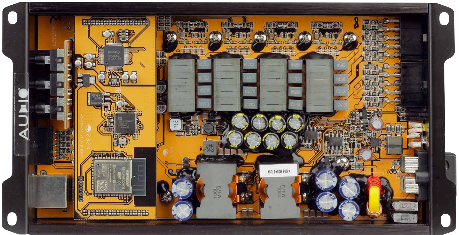
The eight large channels are distributed across four ICs. Each channel has two encapsulated coils and capacitors as a class D low-pass filter
