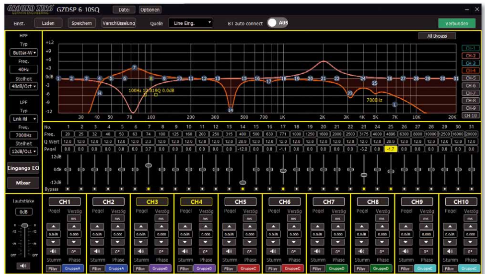
The main window contains almost everything: output EQs, delays, crossovers, volume, etc.
