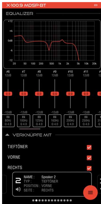
30 fully parametric bands per channel offer all the bells and whistles; the diagram also shows the crossovers
