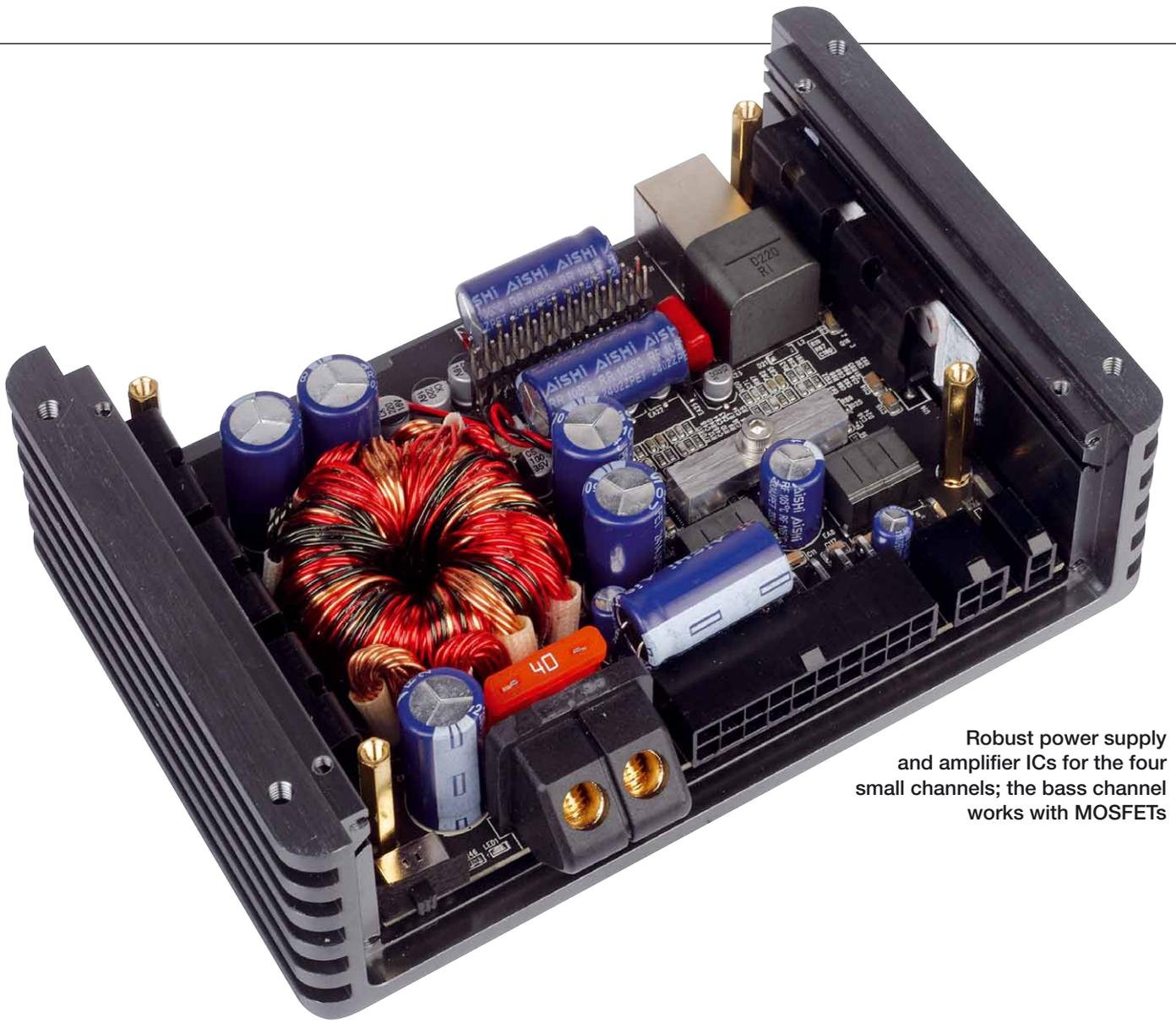
Robust power supply and amplifier ICs for the four small channels; the bass channel works with MOSFETs
