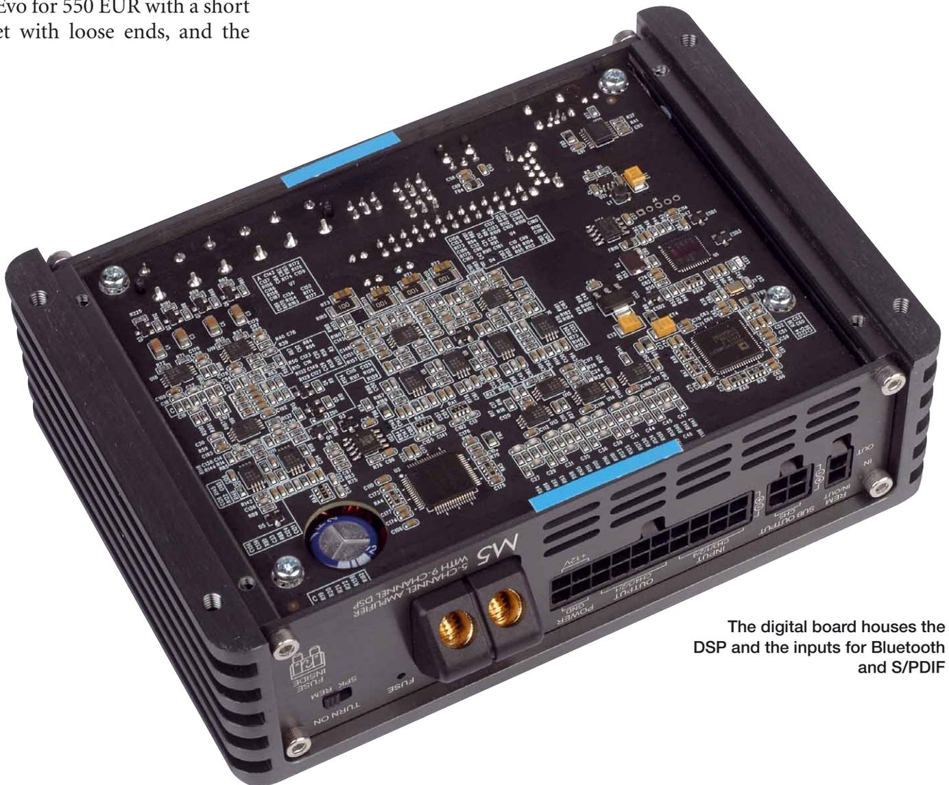
The digital board houses the DSP and the inputs for Bluetooth and S/PDIF
