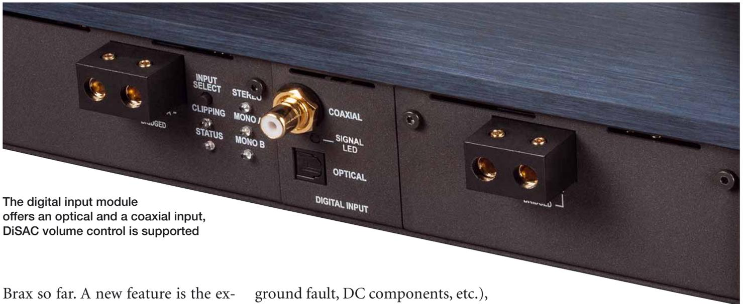
The digital input module offers an optical and a coaxial input, DiSAC volume control is supported
