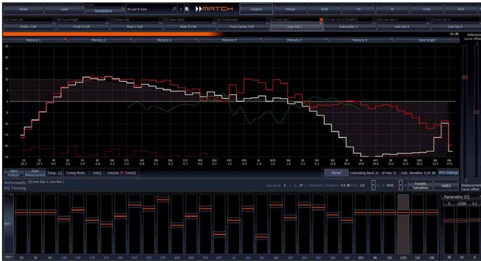
RTA measurement of a mid-range driver: Original curve (red) and result with 24 dB crossing (white). The correction via TuneEQ is shown in green and the EQ bands 4 – 24 are set at the bottom. We measured with an accuracy of 1/6 octave and standard smoothing; it can be finer if desired
