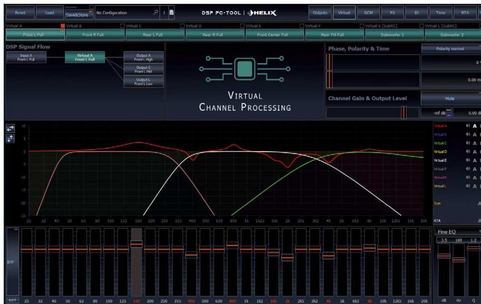
As an alternative to normal routing, Virtual Channel Processing can be used to combine channel groups and equalize them across the crossover frequencies
