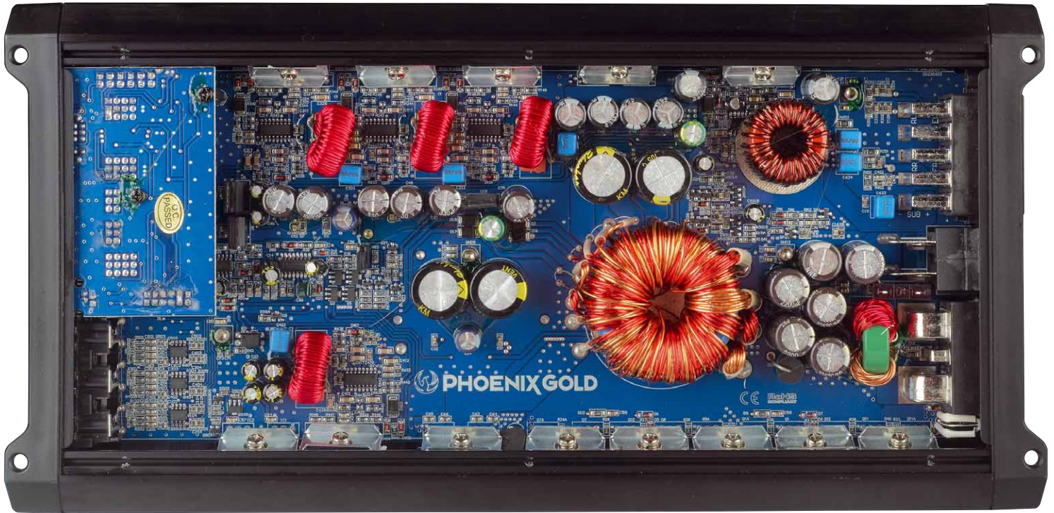
The amplifier paths work with a Class D driver IC and a large-dimensioned toroidal coil
