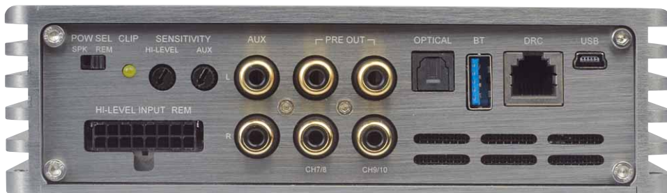
Accessories such as the Bluetooth module make contact via USB. Digital input is also possible via optical S/PDIF
