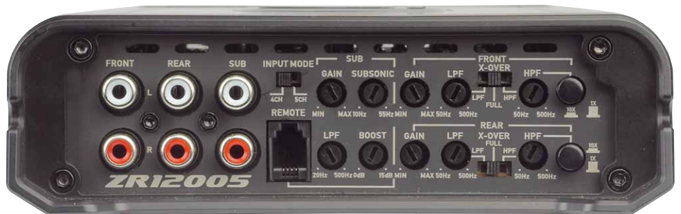
The front panel is packed with controls, and the subwoofer channel has low-pass, subsonic, and boost
