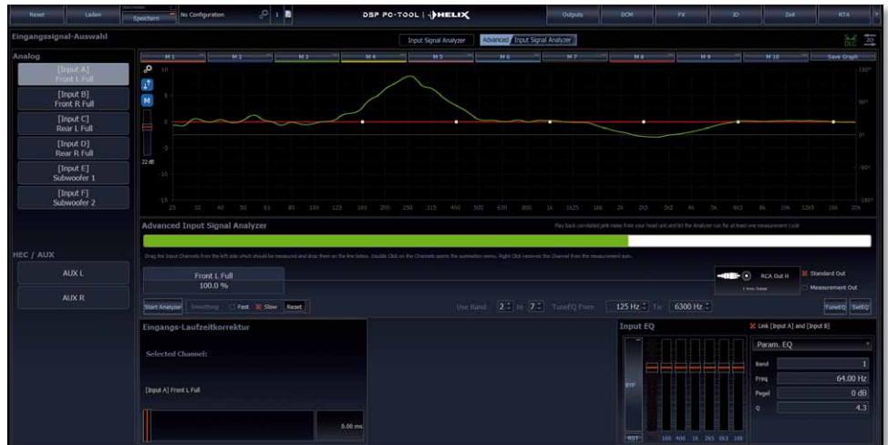
EQ ex works: The measurement of one channel shows a boost and a dip. The curve was zeroed manually
