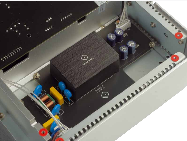
The power supply board with an encapsulated power supply
