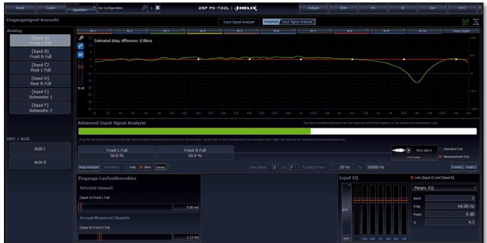
LZK ex works: After the alignment with 1.13 ms, there is still a remainder of 0.06 ms at high frequencies
