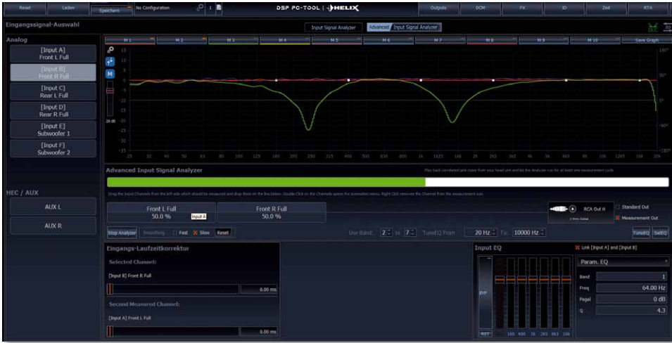
All-pass: In the summation, 2nd order all-passes show up as dips; here there are two of them
