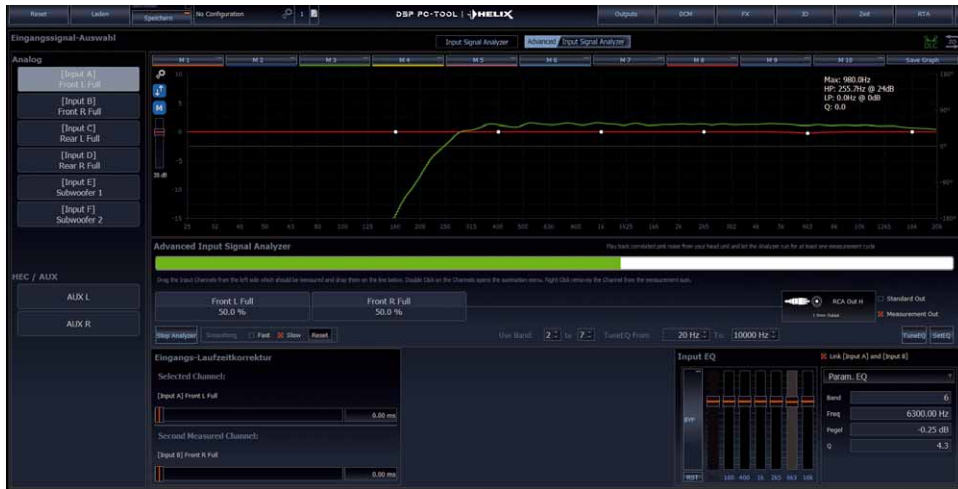
“Display Graph Information” shows the frequency and slope of a set filter
