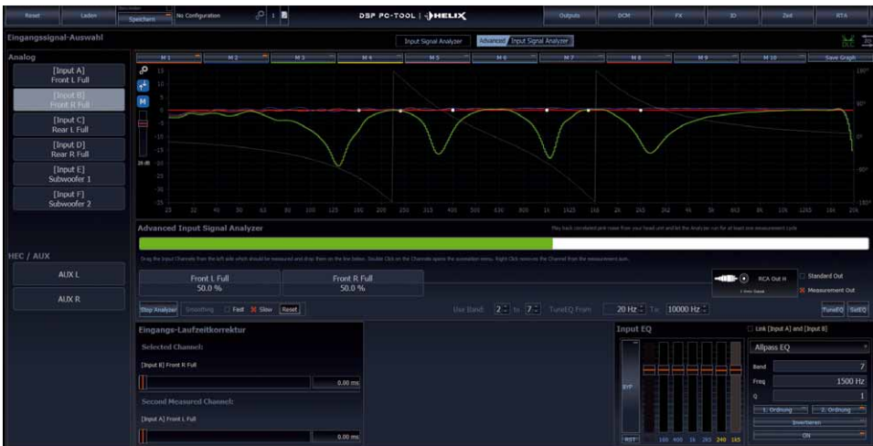
All-pass: If you get the wrong channel during alignment, it gets worse: There are now 4 all-passes instead of 2
