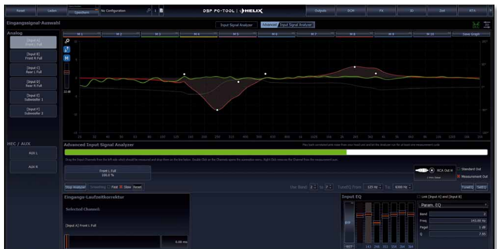
EQ ex works: The control measurement with corrected EQ (green) shows a smooth signal
