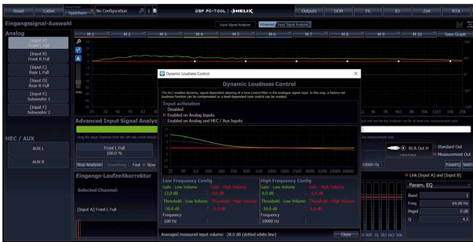
DLC: Finished dynamic loudness setting: Quiet curve (green with +12 dB in the bass, loud curve (red) with -2 dB in the treble, current measurement dotted white
