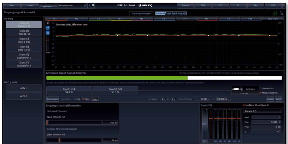
LZK ex works: With the second alignment, the time differences are perfectly equalized, and the sum is smooth
