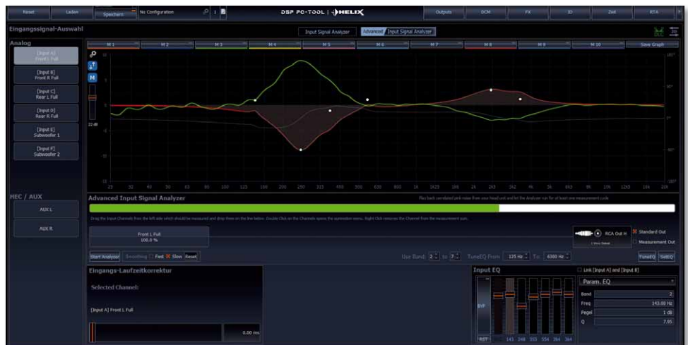
EQ ex works: The TuneEQ presents an alignment with 6 bands from 125 Hz to 6300 Hz, which is then applied with “Set EQ”
