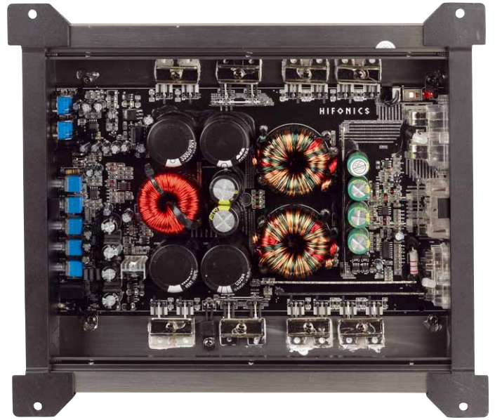
Modern layout with generous power supply inside the mono amp
