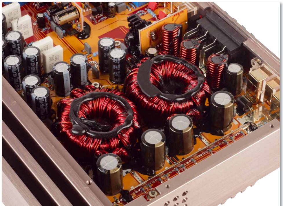
The GZUA 6SQ houses two power supplies, one for the small and one for the large channels
