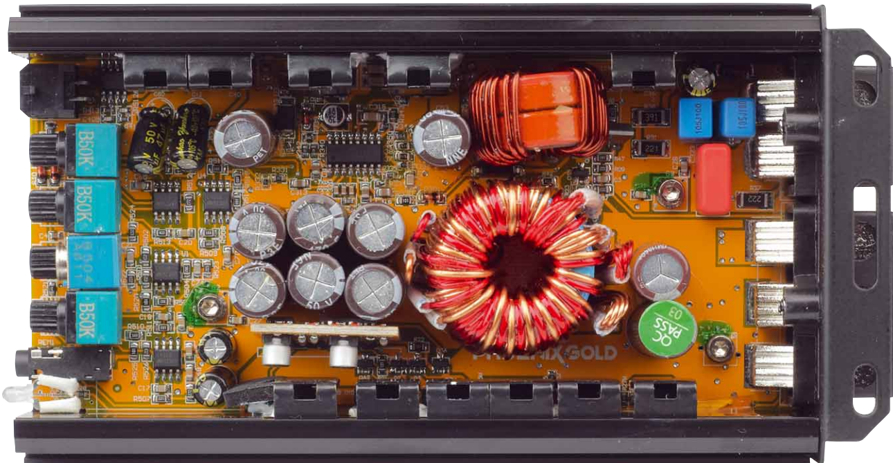
Two large coils can be seen on the PCB: the transformer for the power supply (center) and the standing coil for the class-D filter
