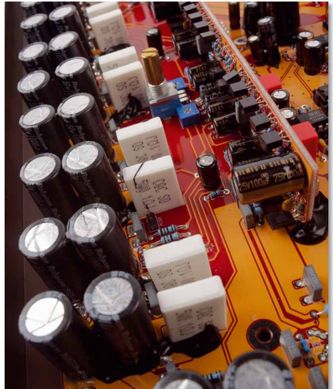
The power MOSFETs are hidden under the PCB. There one pair each for channels 1-4 and two pairs each for channels 5 and 6
