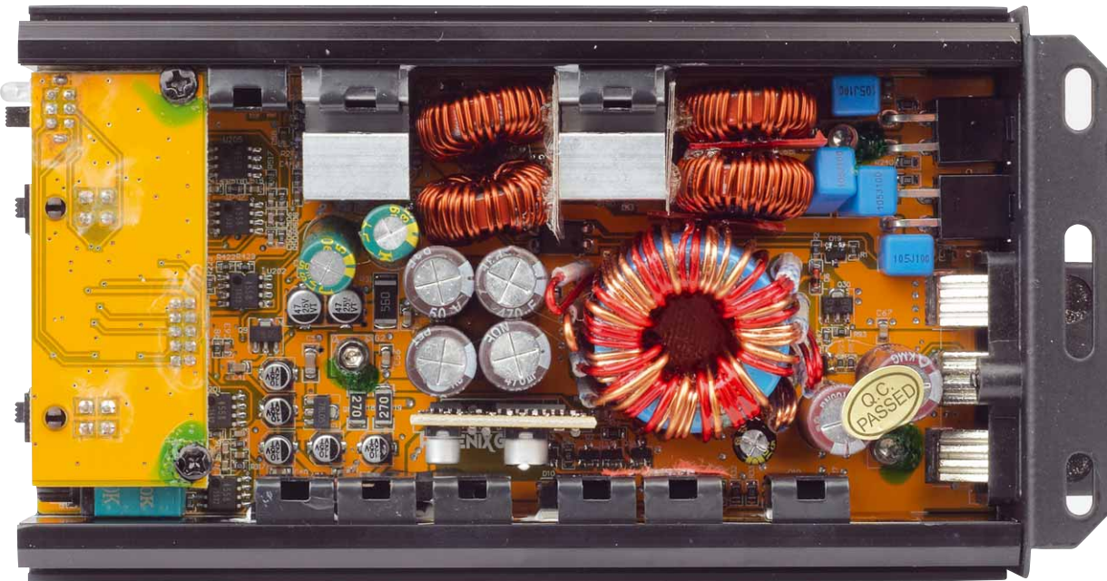
The power amplification is located in the upper part of the PCB, the large components are the two heatsinks and the four class-D coils
