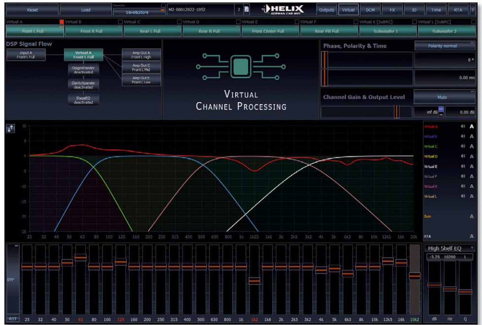
As an alternative to the normal routing, virtual channel processing can be used to combine groups together and equalize them across the crossover frequencies
