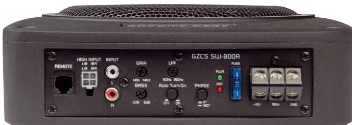
Speaker-level inputs are available as well as a polarity switch, a low-pass filter, and a bass boost
