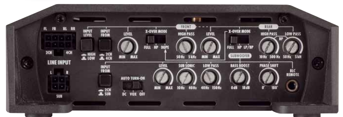
The ZXR has comprehensive filter equipment with a bandpass up to 5 kHz so that it can drive all kinds of loudspeakers
