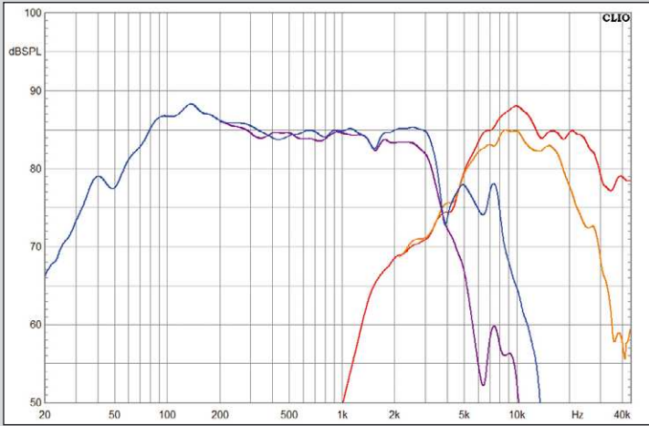
The woofer and tweeter run smoothly both on-axis and under an angle
