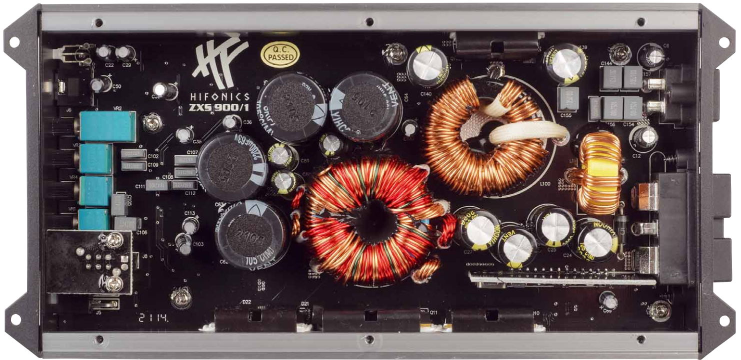
Modern, highly integrated design: mono amplifier with large Class-D inductor (center)
