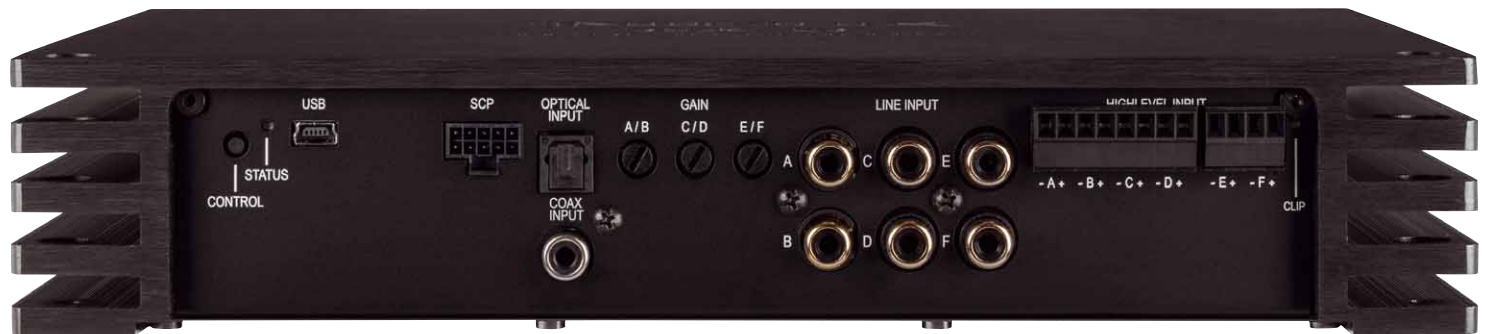
The 6 processed outputs are distributed over 4 RCA sockets and the digital optical output. The inputs feature 6 x RCA, 6 x high-in and digital, either optical or coax
