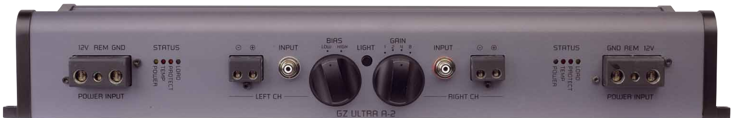
First class wire terminals and RCA sockets and four status LEDs are nice, but mainly the two switches catch the eye
