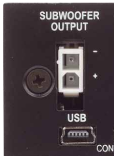
The M 5.4DSP is a full package with Molex sockets, digital input and control port
