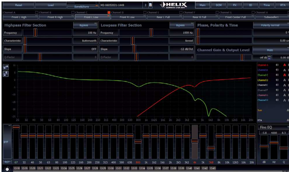
Main window containing crossovers, EQs, time alignment, phase and channel levels
