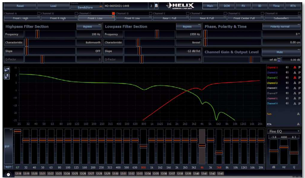
With the HEC BT HD, the PC software DSP PC-Tool can now also be used for wireless programming
