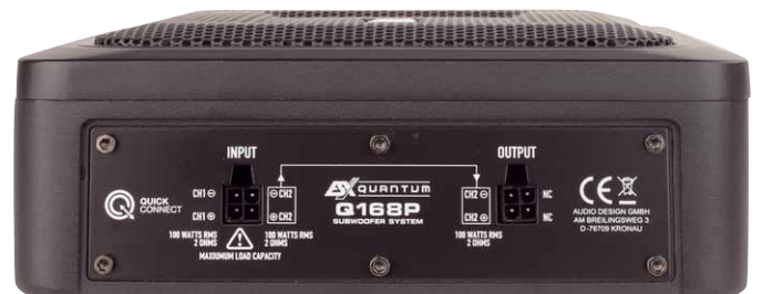
Connection panel with two Molex sockets for amplifier and second woofer
