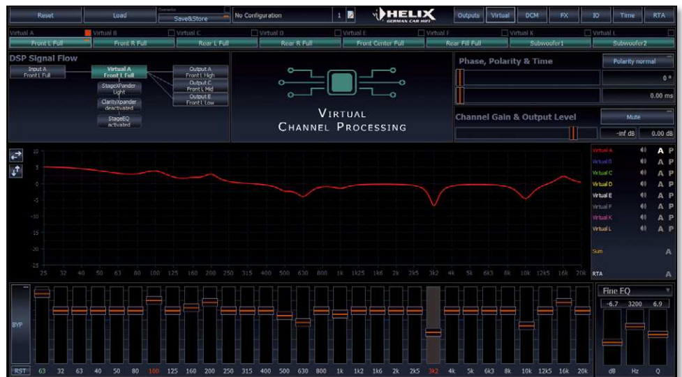
The setup of the virtual channels is similar to that of the output channels, only without crossovers. The virtual front EQ and FX front processing then affect all output channels routed from there
