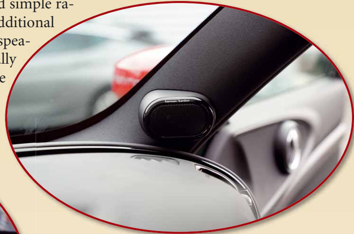
HK system housings were installed to accommodate the Match tweeters
