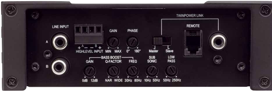
The M ONE X (shown on top) offers plenty of adjustable filters. The M FOUR DSP is fully packed with inputs and outputs
